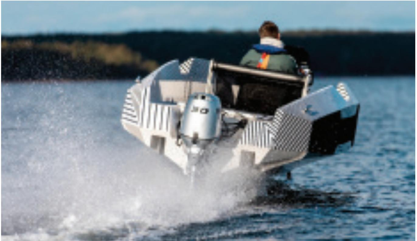
The company decided to go with outboard propulsion, which makes it possible to switch over to electric power as that technology develops.
